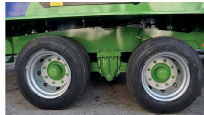
The auto-steer hydraulic rear axle
