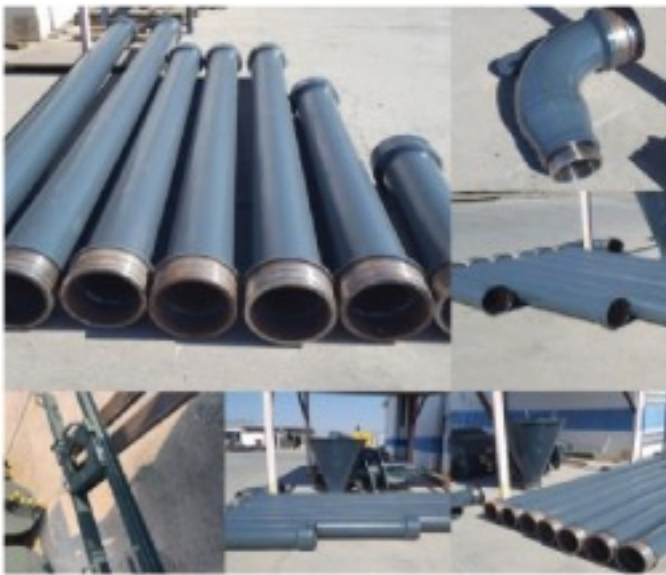
TREMIE PIPE & SPARES
